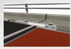
**2.** Where Expansion Joint Assemblies are to be used these should be placed first over the Expansion/movement Joint position.
