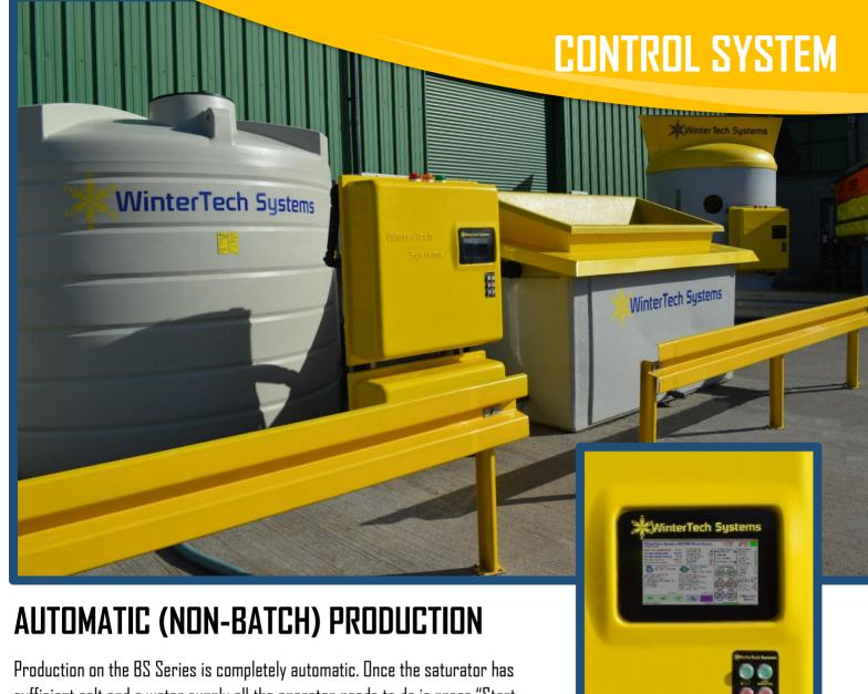
Production on the BS Series is completely automatic. Once the saturator has sufficient salt and a water supply all the operator needs to do is press "Start Production". From here the control system will handle the rest. Brine production begins with the control system dissolving the salt crystals. The brine at this stage is in an unprocessed state and is at about 26-27%
