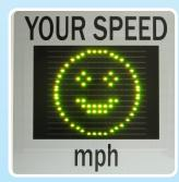
TruSign uses a built-in radar to measure vehicle speeds. Speeds above a user-defined threshold are displayed, along with a range of pictograms and messages if required. Pictograms include warning signs for sharp bends, cross roads or roundabouts. Messages include warnings such as Slow Down or Too Fast. Tru-Sign can display the speed only, or the speed alternating with a message or pictogram.
