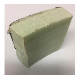
iLine with its partner JBA Consulting designed a high-strength GRP / UV CIPP liner with an effective diameter of 1500 mm. The liner thickness was 30 mm and the difference here no one worldwide had produced or installed a UV liner of that thickness before.
