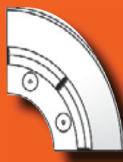
RediKerb SP 180 degree Corner Unit 250mm Radius 125mm high 7.7kg weight 4 Fixings
