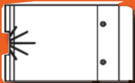
BusPad Ramp Module 750mm wide x 500mm long 65mm high 16.0kg weight
