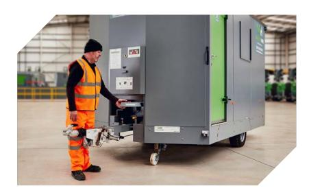
Our unique, retractable drawbar results in up to 40% smaller footprint once in place onsite compared to other mobile welfare units on the market. This space saving affords greater flexibility for locating onsite, as well as minimising trip hazards and potential damages with optimal HSE compliance.
