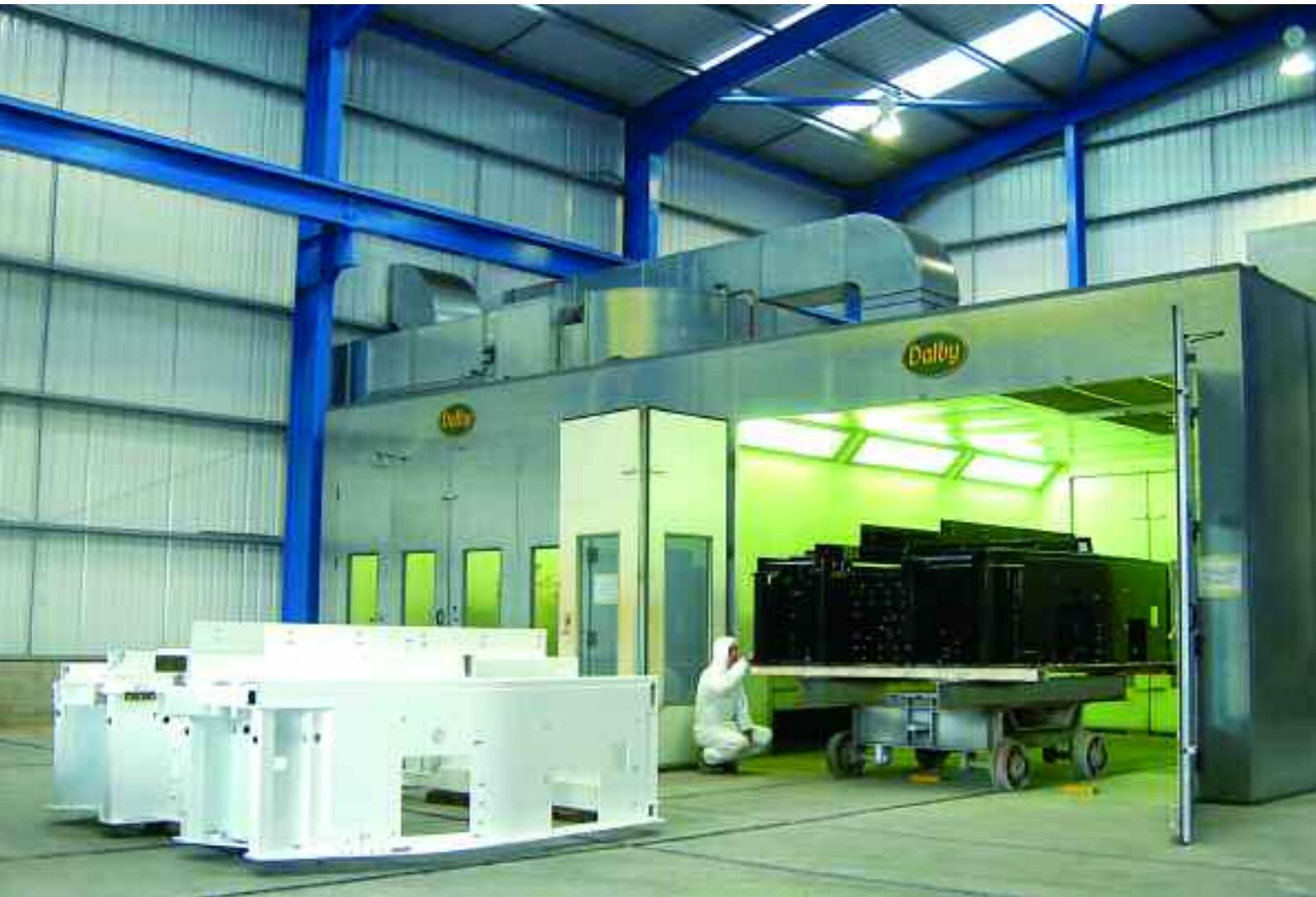
Tandem spray bake booths, provide additional flexibility
