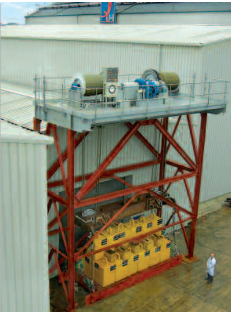
Gate hoists for hydro-electric project, works assembly and load testing | Nathpa Jhakri, India
