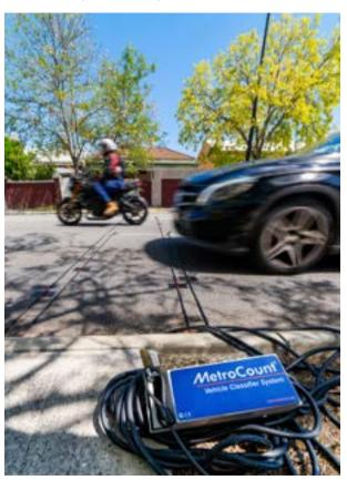
The RoadPod® VT4 is the solution for collecting comprehensive and accurate data from multi-lane roads, often used for monitoring highways.
