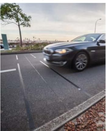
The RoadPod® VP offers the highest level of accuracy and detail for a permanent monitoring solution. Designed for multi-lane data collection, the system uses two low profile piezoelectric strips embedded in the pavement.
