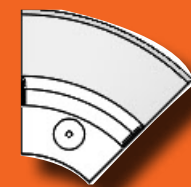
RediKerb SP 135 degree Corner Unit 250mm Radius 125mm high 5.8kg weight 3 Fixings
