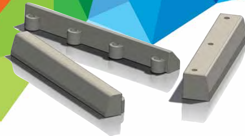
RediKerb SP Straight 150mm wide x 1000mm long 125mm High 10.5kg Weight 4 Fixings
