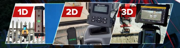
1D dig depth system includes rotating laser and receiver mounted on dipper stick with or without in cab display. 2D dig depth and length of excavation system includes sensors fitted to bucket, stick, boom and chassis with in cab display. 3D dig depth, length and positioning of excavation system includes sensors fitted to bucket, stick, boom and chassis with in cab display. Plus, the addition of GPS receivers, modem and compass enables positioning and 2-way data transfer.
