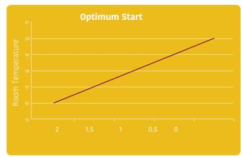
temperature rise are non-adjustable. The optimisation process will be cancelled if any overrides are used during the 2-hour period of operation.
