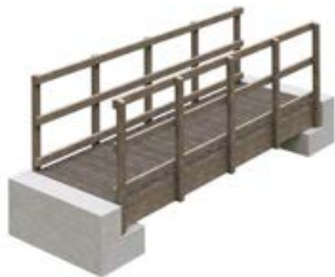
Existing abutments can be used. They may not always be concrete. Soil may need to be retained.
