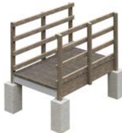
Other methods of abutment can be incorporated. This includes posts, screw piles, gabion baskets and stabilised soil methods.
