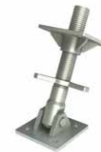
Adjustable Pivot End Compression = 210kN* Tension = 85kN *prop length at 3m
