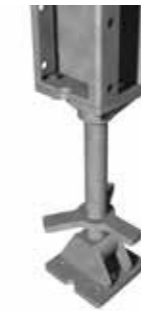
Adjustable Pivot End Compression = 100kN Tension = 65kN
