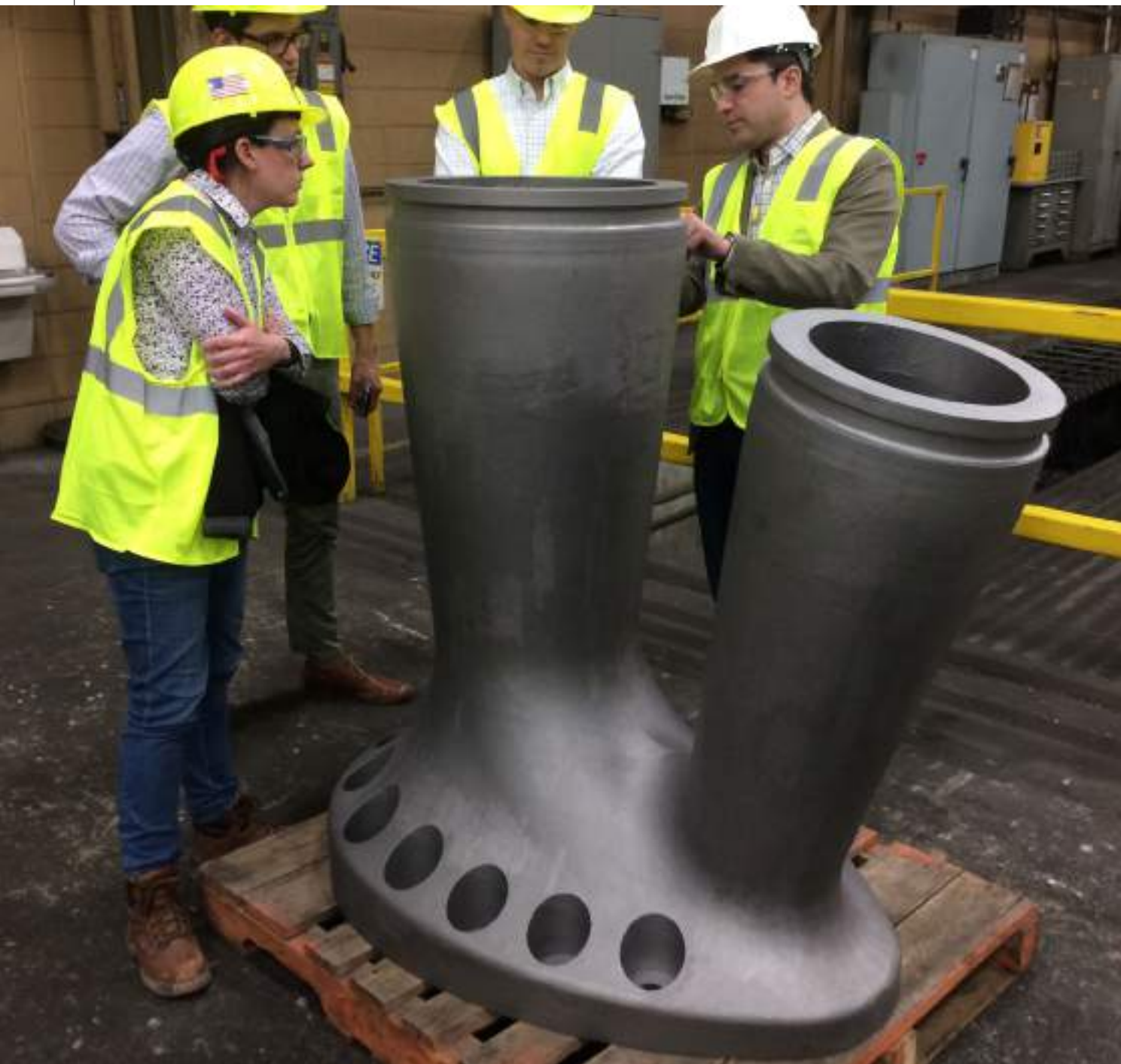
Custom cast steel node designed for an expansion at Charlotte Douglas International Airport
