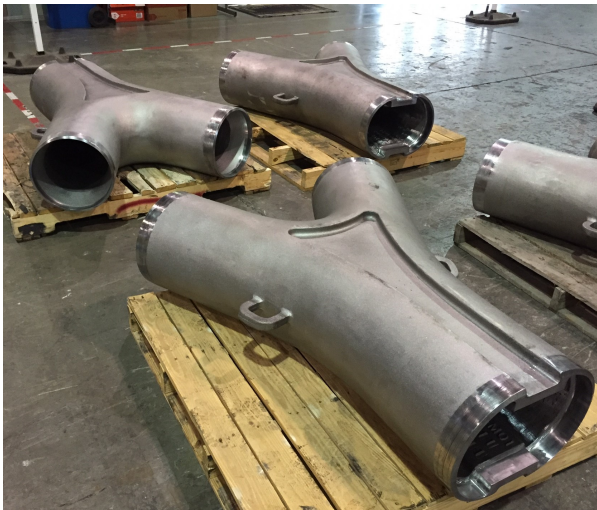
Figure 8: Cast steel nodes for the Frances Appleton Pedestrian Bridge awaiting incorporation into the bridge pier assembly at the fabrication shop. Machined weld preps support shop assembly and improved tolerances. AESS weld remediation is limited to three, simple girth, shop-welds. The recessed detail was precision machined to meet the architectural requirements.
