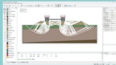
**+** DLO analysis quickly identifies the critical collapse state
