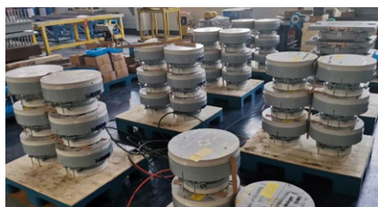
Spherical bearings with clamps for non-frequent uplift forces
